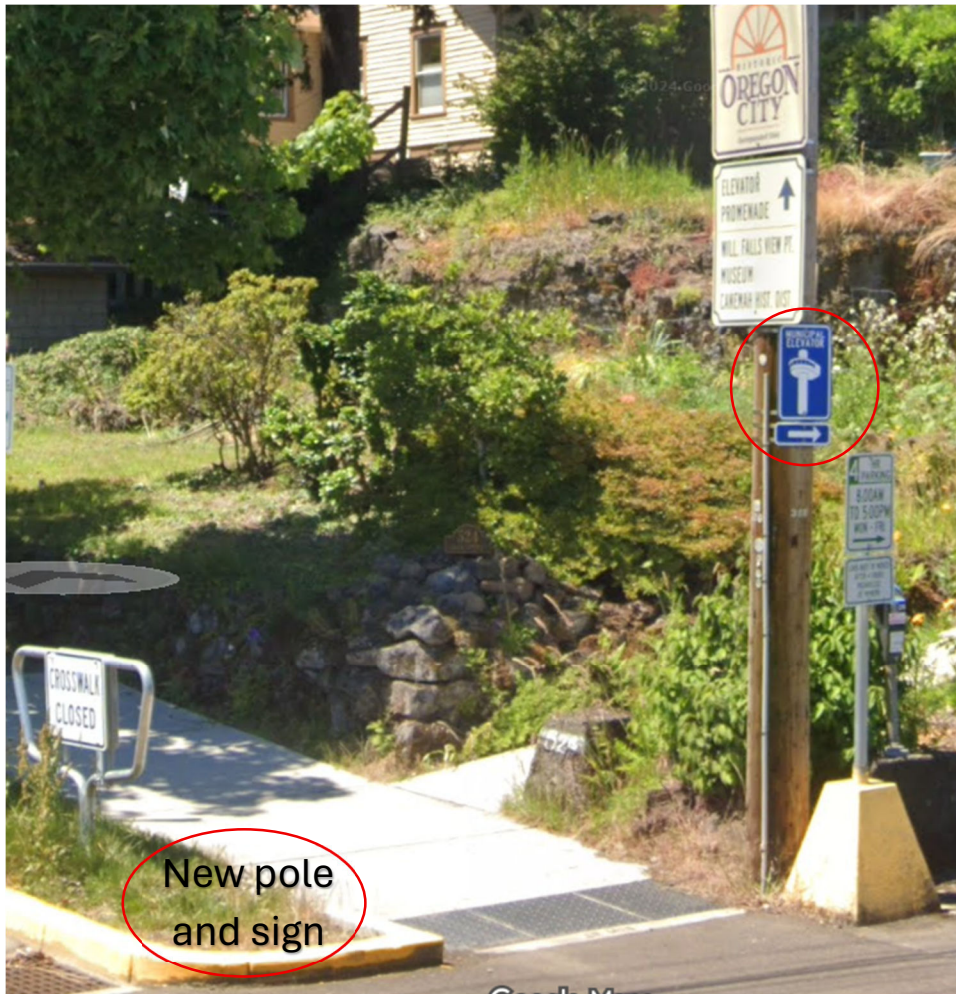
Figure 2: Location 1 – Remove existing blue sign and add new sign on a new black pole to match location 2.
