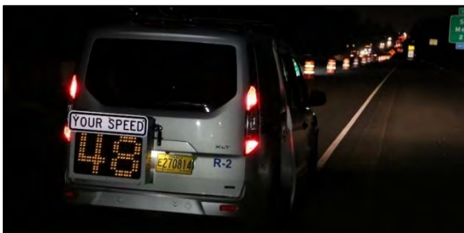
Figure 500.4-1: Mobile Photo Radar in a Medford Work Zone
