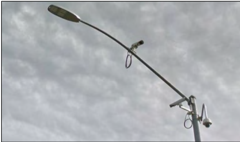
Figure 500.4-4: Examples of Cameras Used for Traffic Operations, Not Enforcement
