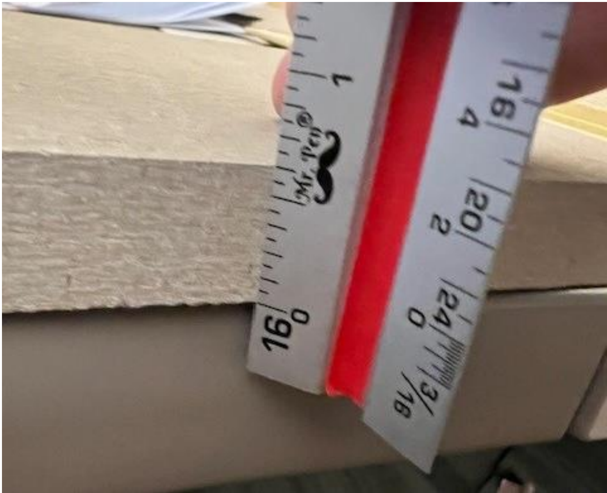
Sample A showing 0.625-inch thickness
