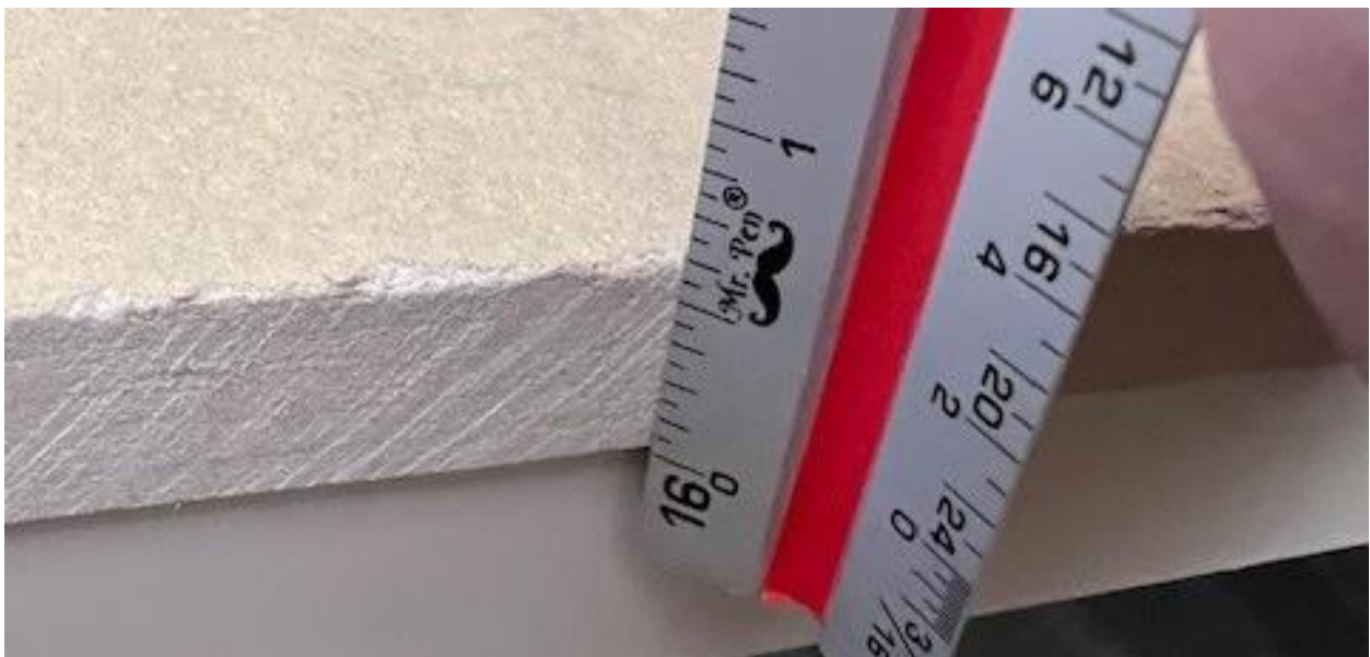
Sample C showing 0.625-inch thickness
