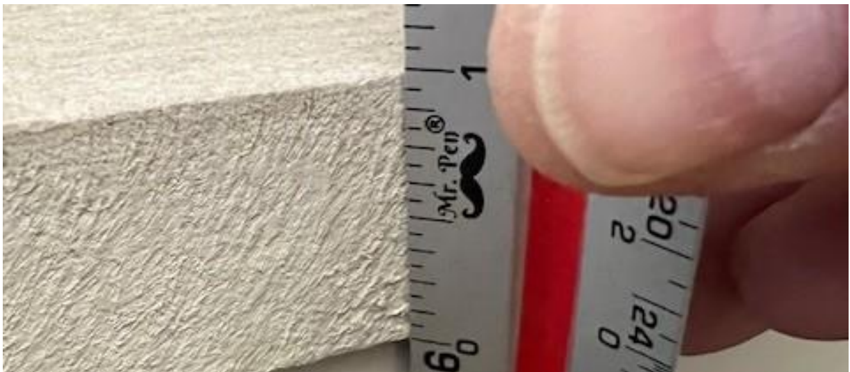
Sample fiber cement corner board showing 1-inch thickness
