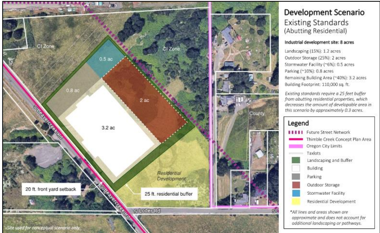
Figure 4. Development Scenario – Existing Standards (Abutting Residential)
