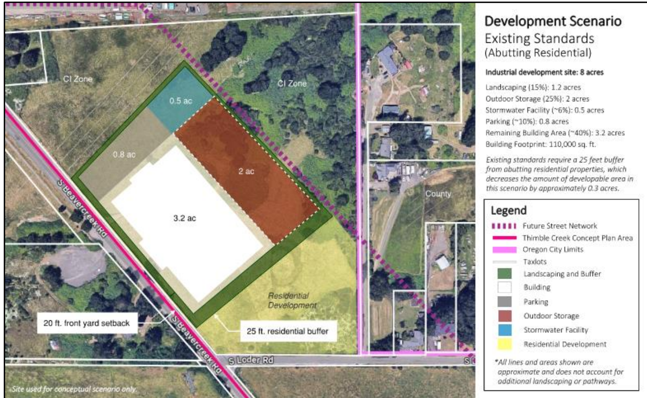
Figure 4. Development Scenario – Existing Standards (Abutting Residential)
