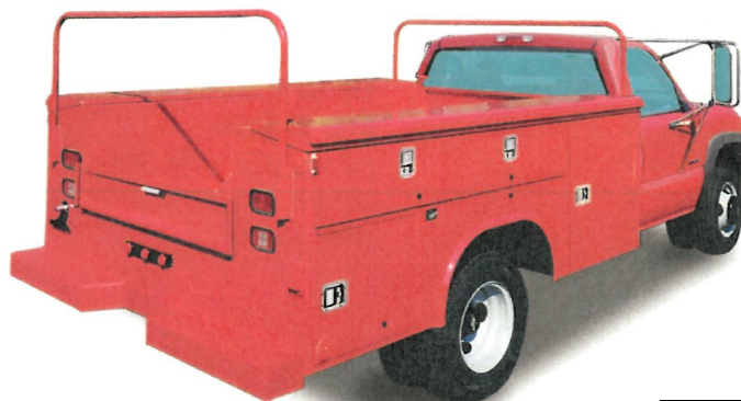
Spacemaker Low Profile Service Body SLP108DW ("B" side shown) Model shown features Spacemaker compartments with recessed tail lights, optional removable overhead ladder rack, and deck plate step bumper with recess
