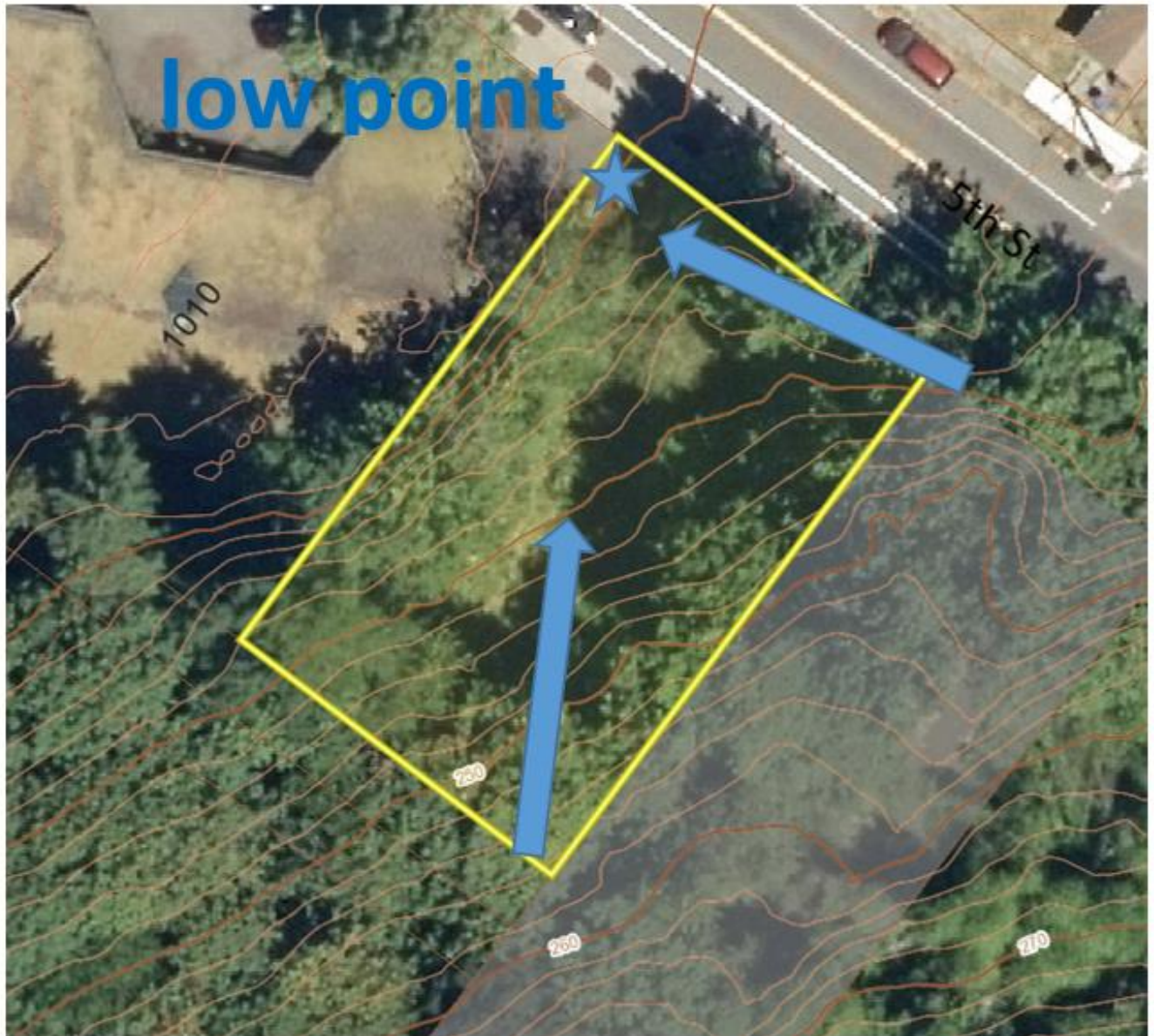
Figure 2- Aerial phot and topography- arrow showing cross- slope
