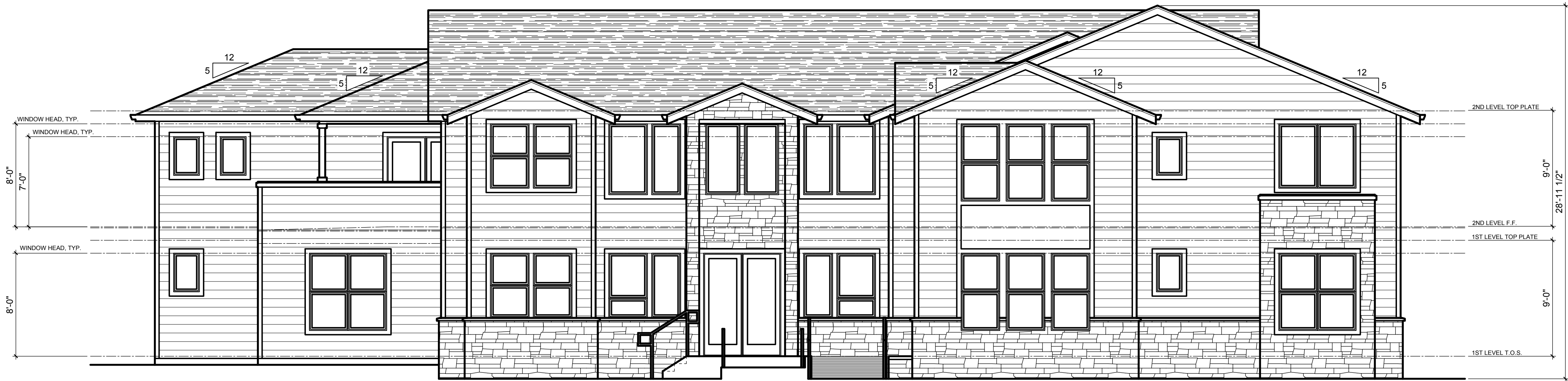
A FRONT ELEVATION (NORTH) A2.0 SCALE: 3/16" = 1'-0"
