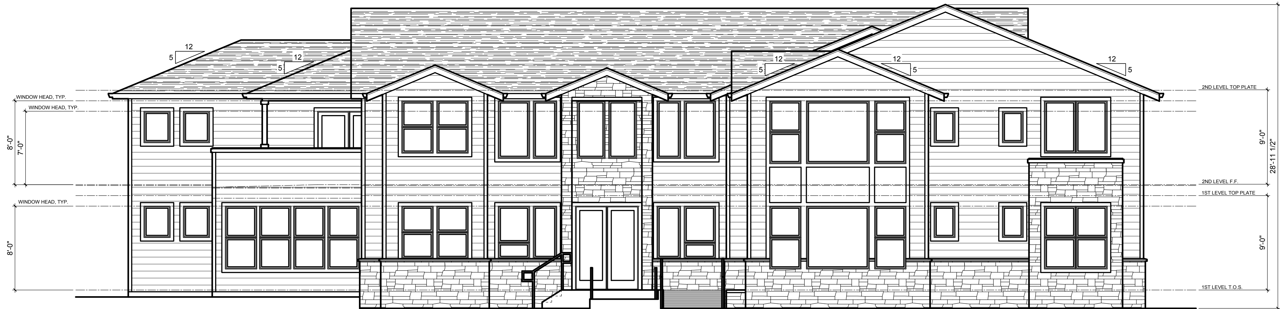
A FRONT ELEVATION (NORTH) A2.0 SCALE: 3/16" = 1'-0"
