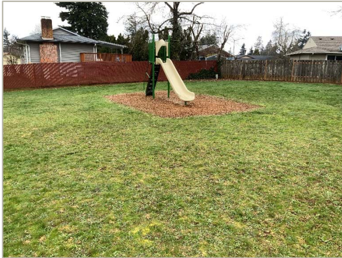
3 – NO ACCESSIBLE PATH TO PLAY STRUCTURE
