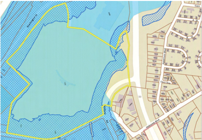
Figure 2.3 - FEMA 100-yr floodplain and the 1996 Flood Inundation
