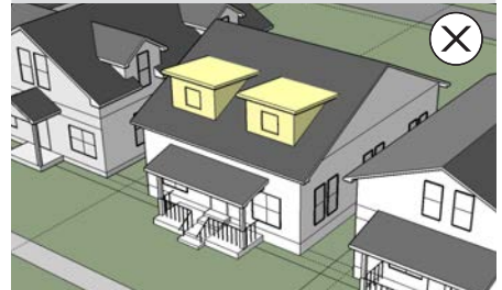
2. The new dormers illustrated above on the front-facing roof plane are inappropriate because they have shed roof style that is not seen in the surrounding historic context and visually overwhelm the original roof.
