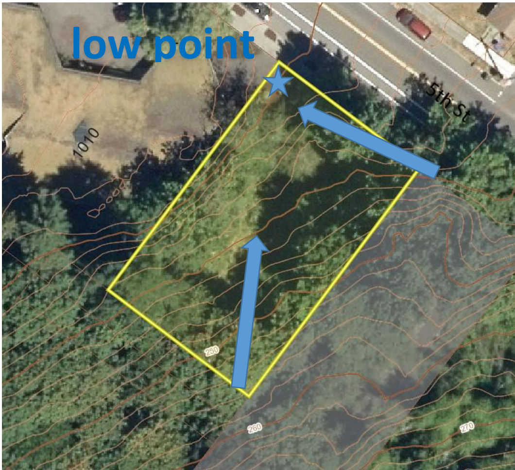
Figure 2-Aerial photo and topography- arrow showing cross-slope
