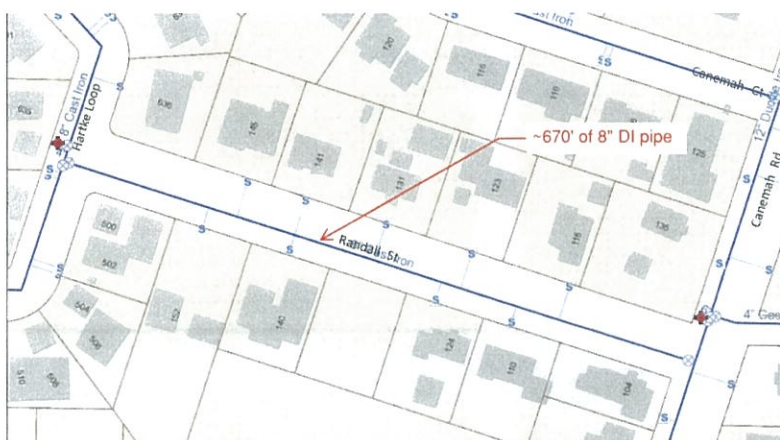
5. Randall Street - Waterline Replacement
