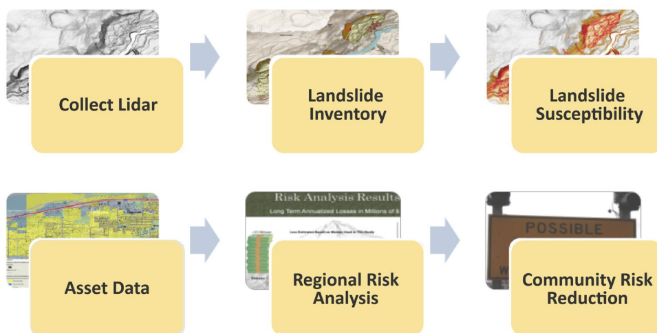
Figure 3-2. Landslide Risk Reduction Process Overview
