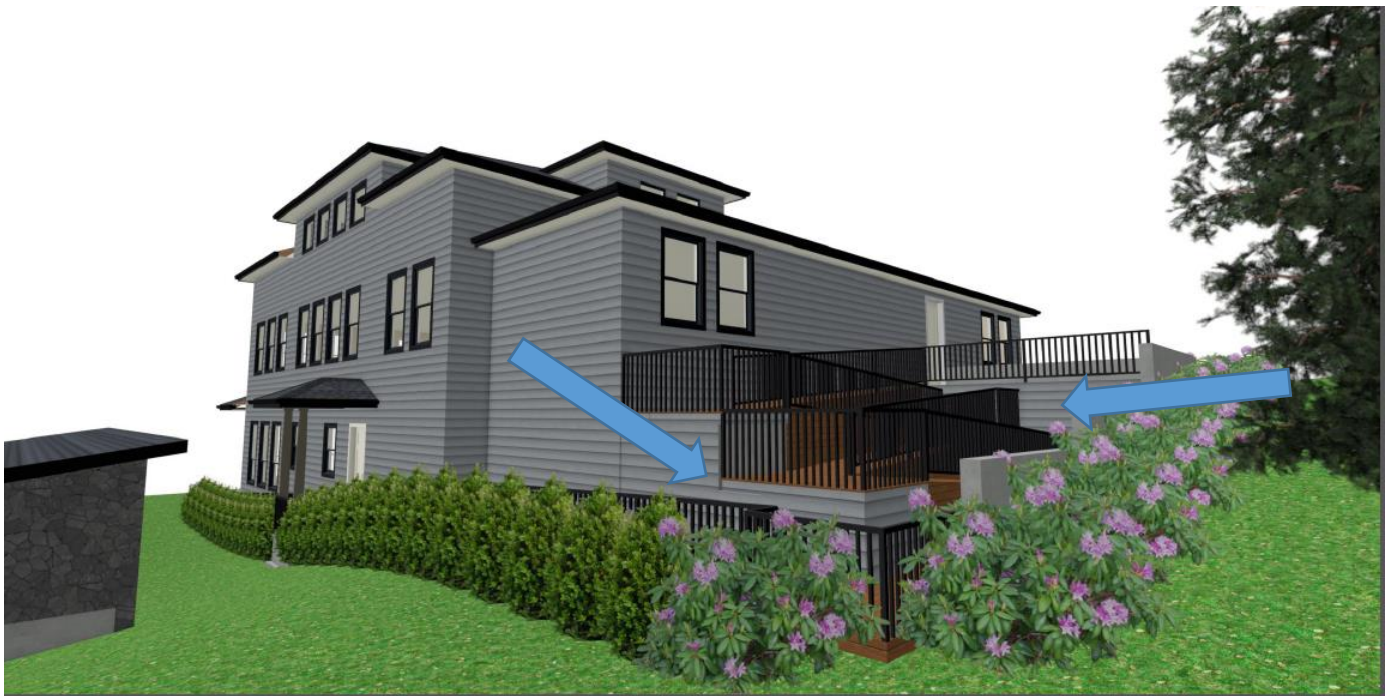
Figure 20- Side (right) and rear rendering. The blue arrows highlight highlights the areas addressed in the recommended revisions that require the removal of all horizontal siding from ADA ramp. ** NEW METAL RAMP DESIGN **
