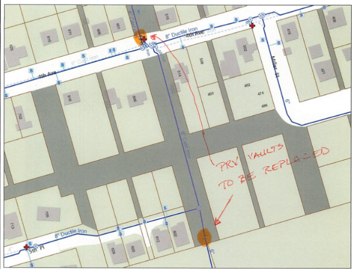
Project A: 4 th Ave. and 5 th Place PRV Replacement
