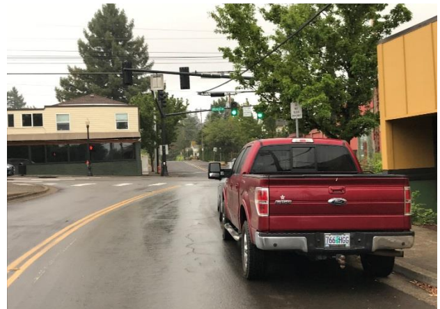
Figure 3. Image Showing Limited Visibility of Intersection and Crosswalk due to On-Street Parking (Westbound on Pearl Street)
