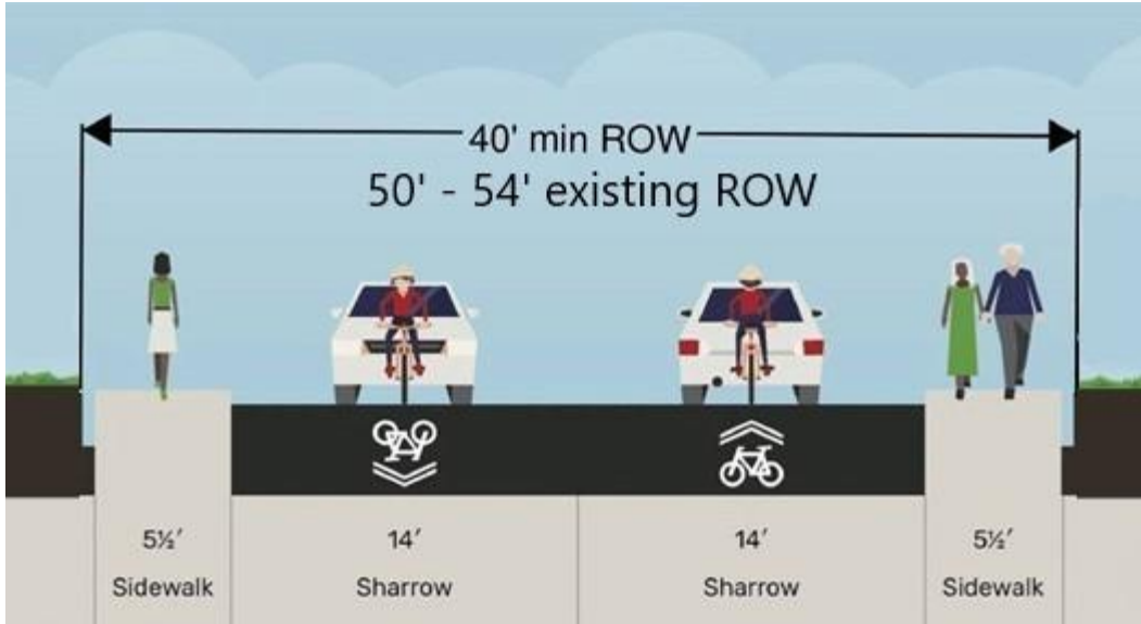
Figure 4-3: Apperson Street Cross Section
