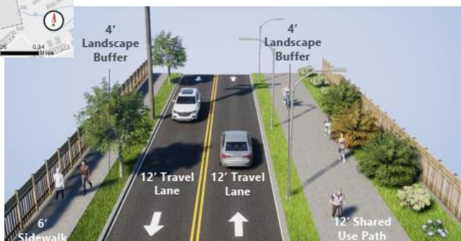
Figure ES-5. Meyers Road Cross-Section
