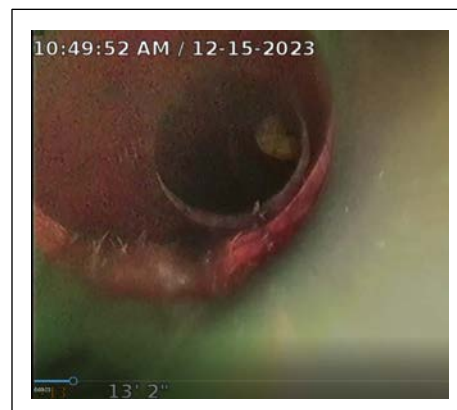
Tree root intrusion in pipe
